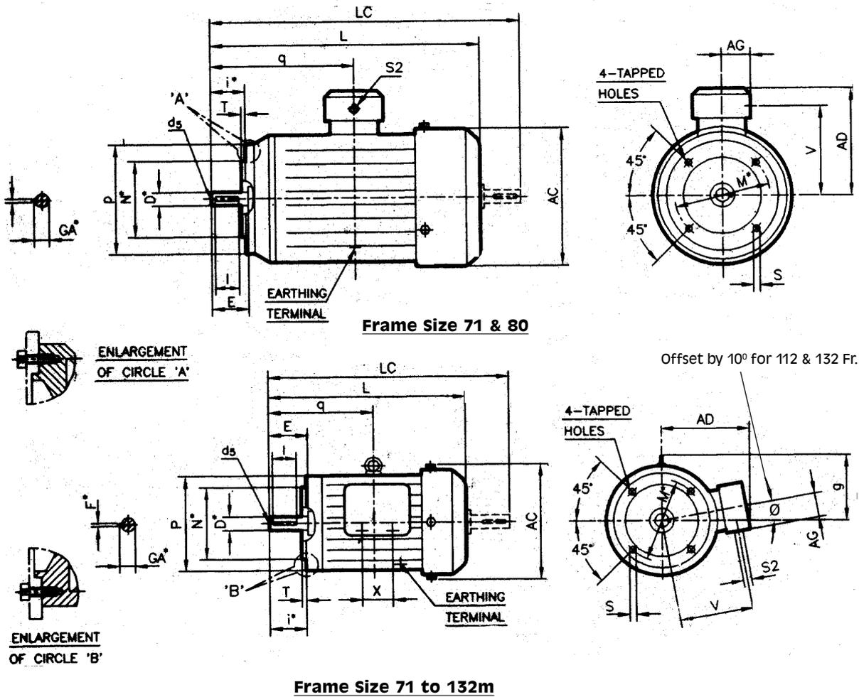
**Dimensional Details : Face Mounted (B14 Construction) TEFC Standard Brake Motor Frame 71-132M**
