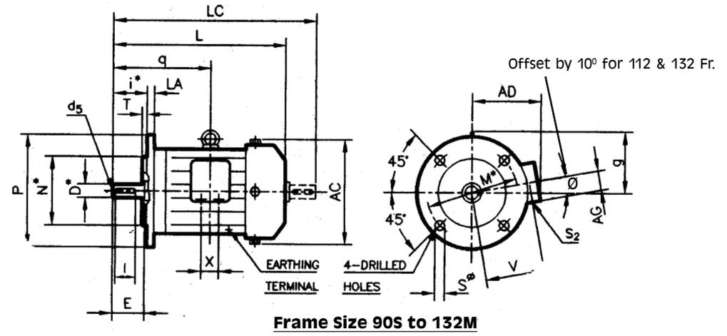
**Dimensional Details : Flange Mounted (B5 Construction) TEFC Standard Brake Motor Frames 71-132M**
